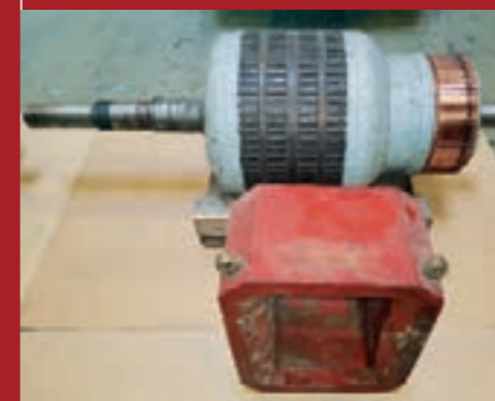
Original design: Rotor and field coil from 1900
