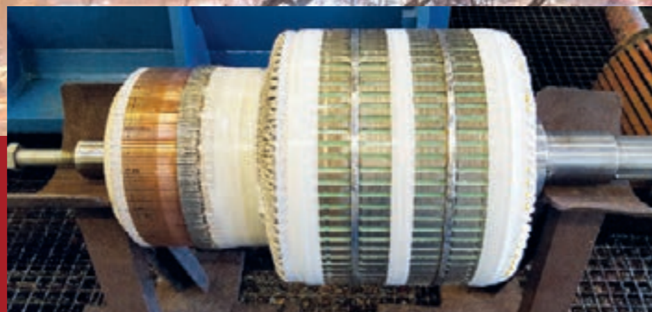
Rotor winding before vacuum impregnation with visible steel straps
