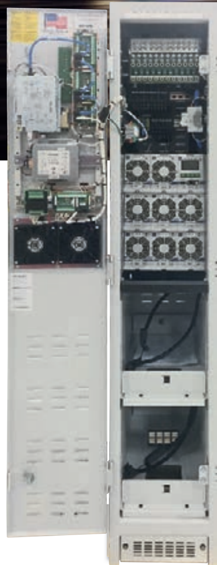
Slim Power System with 3000 HD Rectifier (9kW @ 48V DC) and HDi DC Converters (3kW @ 24V DC) for installation into restricted space locations for Public Safety Radio Systems
