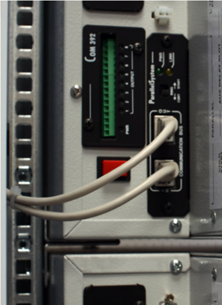
Parallel configuration and programmable relay contacts board
