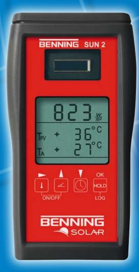
BENNING SUN 2 – Insolation and temperature measuring instrument for photovoltaic systems and solar thermal systems
