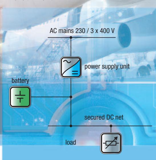
Fig. 2: Standby parallel operation
