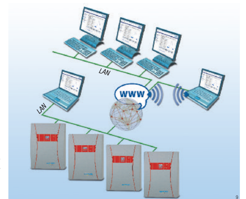
System monitoring communication possibilities
