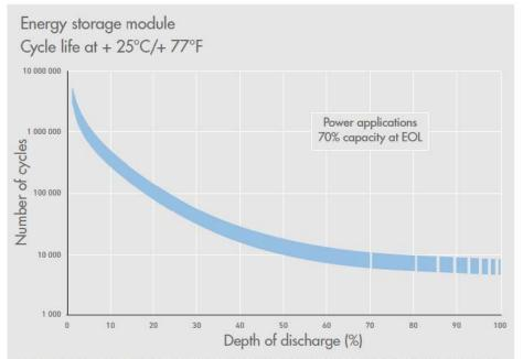
Cycle life depends on both depth of discharge (DOD) and charging rates. The above results are based on testing at a fixed DOD and varying charging rates. The end of life (EOL) is reached when the remaining capacity is 70% of the initial capacity.
