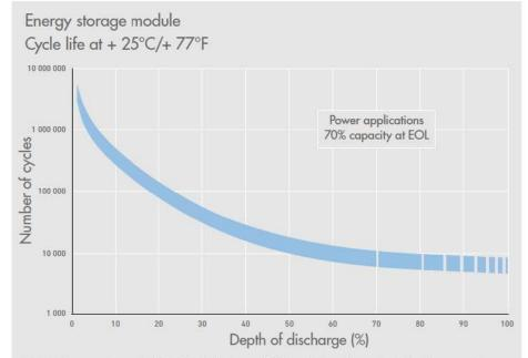
Cycle life depends on both depth of discharge (DOD) and charging rates. The above results are based on testing at a fixed DOD and varying charging rates. The end of life (EOL) is reached when the remaining capacity is 70% of the initial capacity.
