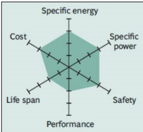
Although moderate in overall performance, newer designs of Li-manganese offer improvements in specific power, safety and life span.
