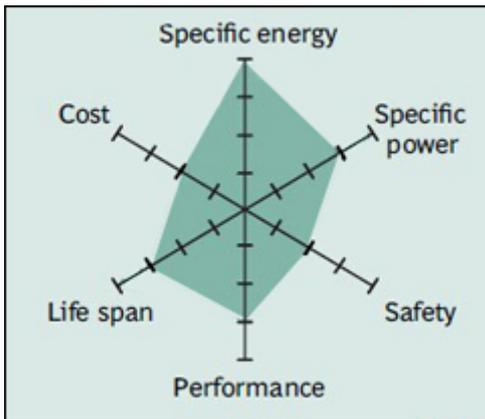
High energy and power densities, as well as good life span, make NCA a candidate for EV powertrains. High cost and marginal safety are negatives.
