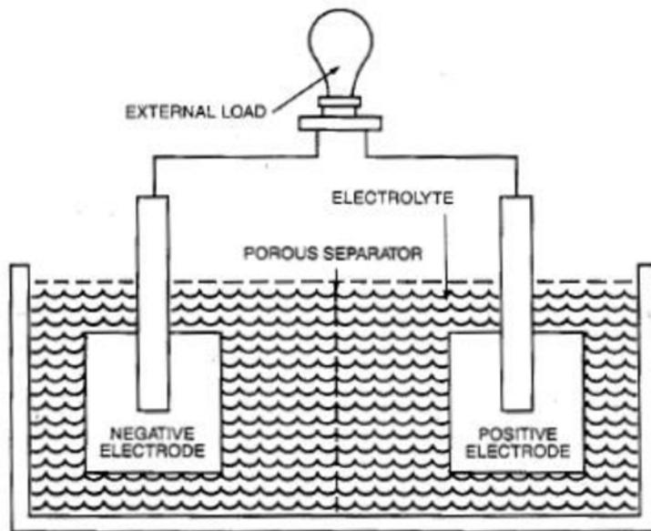
The battery separator is an essential component of batteries that strongly affects their performance. The control of their properties being particularly important for obtaining lithium-ion batteries with high cycling performance. Separators are placed between both electrodes, should show high ionic conductivity, excellent mechanical and thermal stability.
