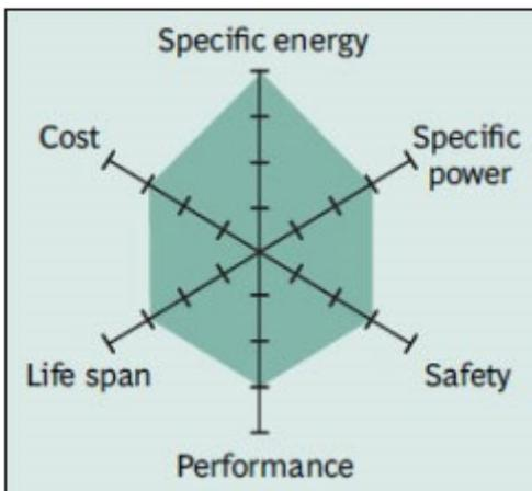
NMC has good overall performance and excels on specific energy. This battery is the preferred candidate for the electric vehicle and has the lowest self-heating rate.
