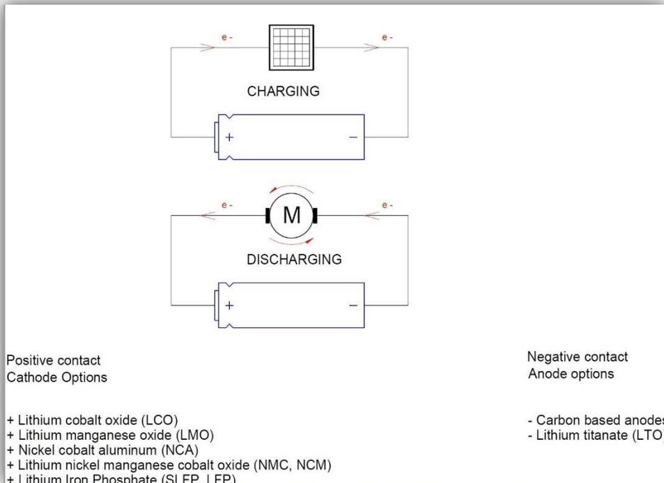
Cells convert chemical energy into electrical energy (and vice-versa). In Lithium ion batteries, during cell charge, the lithium ions flow from the cathode to the anode and they are stored there. During cell discharge, lithium ions disassociate from the anode and flow to the cathode through the electrolyte and electrons are transported by the external circuit to do an effective work.
