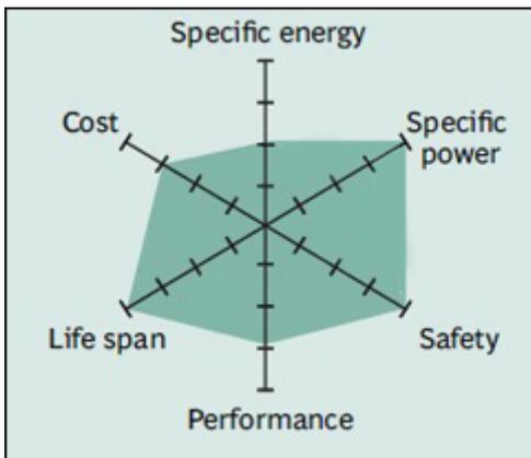
Li-phosphate has excellent safety and long life span but moderate specific energy and elevated self-discharge.
