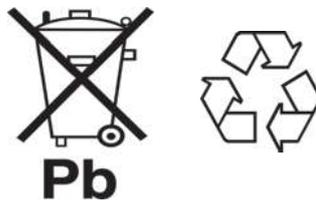
In addition Lead-Acid batteries have to be labelled with the hazard symbols described below:
