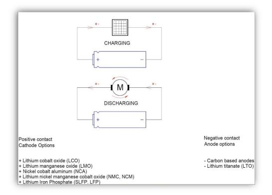
Cells convert chemical energy into electrical energy (and vice-versa). In Lithium ion batteries, during cell charge, the lithium ions flow from the cathode to the anode and they are stored there. During cell discharge, lithium ions disassociate from the anode and flow to the cathode through the electrolyte and electrons are transported by the external circuit to do an effective work.
