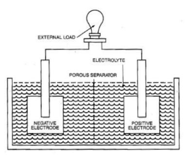
The <u>battery separator</u> is an essential component of batteries that strongly affects their performance. The control of their properties being particularly important for obtaining lithium-ion batteries with high cycling performance. Separators are placed between both electrodes, should show high ionic conductivity, excellent mechanical and thermal stability.
