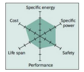
Although moderate in overall performance, newer designs of Li-manganese offer improvements in specific power, safety and life span.
